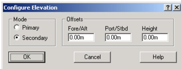
Assign the vehicle's height or depth by selecting the Primary or Secondary radio button on the dialog. In the Vehicle Text window, a vehicle's elevation (ELEV) will have the opposite sign of its depth (ROV D). The Height offset will be subtracted from the observed value. All the offsets are used for pitch and roll corrections.
